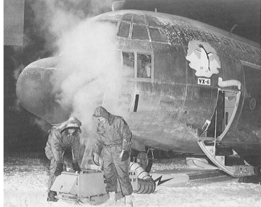
Personnel pre-heating C-130, BUNO 148321 at McMurdo, prior to takeoff for the first winter medevac from Byrd Station in April 1961.
