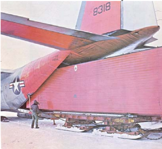
The Plateau Station vans were designed to fit snugly inside the LC-130. This van will be connected to others by roof and floor creating extra space for work and relaxation.
