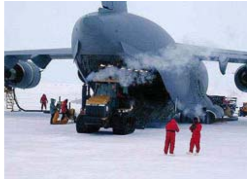
A Challenger 95 emerges from a U.S. Air Force C-17 cargo aircraft. The vehicle will be used during the upcoming Antarctic research season.
