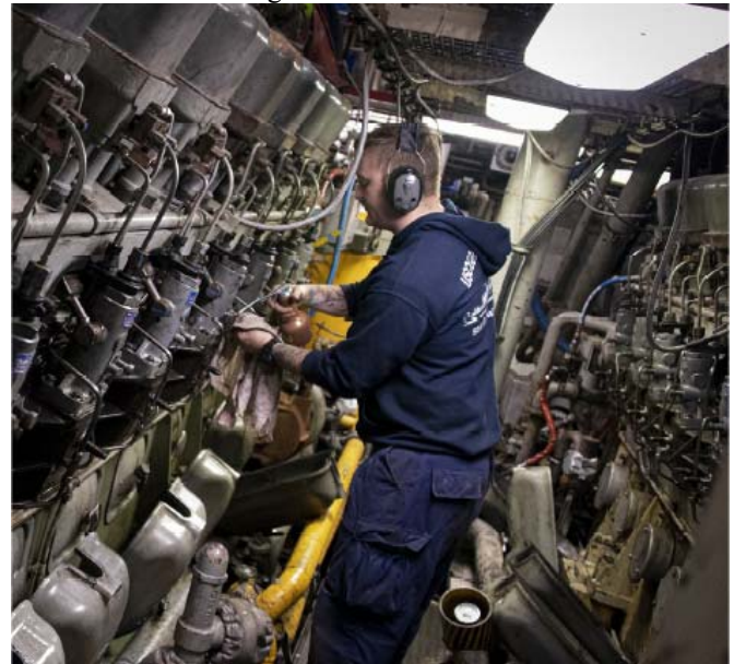
U.S. Coast Guard Fireman Derrek Bost oils parts of an engine on Polar Star about 800 miles north of McMurdo. The Polar Star is equipped with nine diesel engines, which provide 75,000 horsepower to break the ice near Antarctica.
