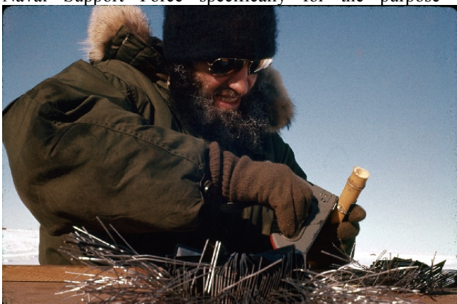
Henry Preparing snow accumulation stakes to set out at mile markers on the Byrd to Pole traverse
