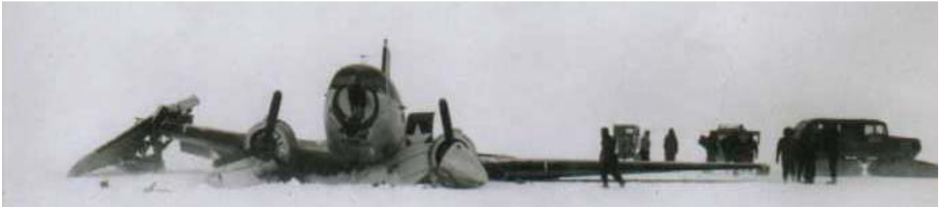
On Christmas Eve 1959 R4D-8 (Buno 17154) crashed while attempting a landing in a whiteout at Byrd Station. Lieutenant Garland M. Regenar was on final approach when the Dakota stalled and the right wing dropped. Although Regenar applied power and used his rudder to compensate, the right wing hit the surface and broke. There were no injuries, but the aircraft was destroyed.
