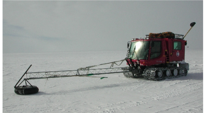
In 2002 This PistenBully Was Adapted For Crevasse Detection Using a 20 Foot Boom Extension With An Inner Tube At It's End. The Ground Penetrating Radar Antenna Rests In The Inner Tube.
