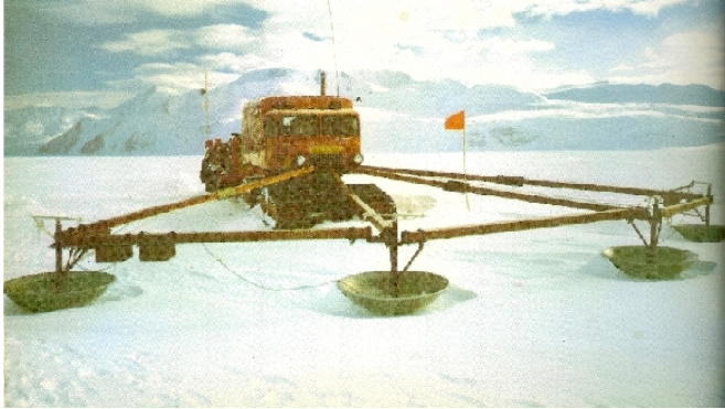
In The Early 1960s Vehicles Like This Sno-Cat Moving Through The Mountains Of Victoria Land With It's Crevasse Detector Out In Front Like Outstretched Fingers Was Used To Explore The Continent
