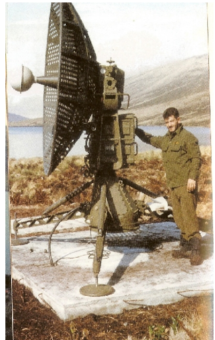
ET3 Johnnie Vito Working on the Rawinsonde (GMD). The GMD was donated to the New Zealand Meteorological Service by the US Navy to obtain weather information for the Deep Freeze flights between New Zealand and McMurdo. The GMD originally was used in Korea by the US Army and it had not been inspected or tested before being shipped to Campbell Island. Vito was scheduled to winter-over at Byrd Station and he was detoured to Campbell Island to help install and to repair the GMD. As it turned out he was there for most of the summer season.
