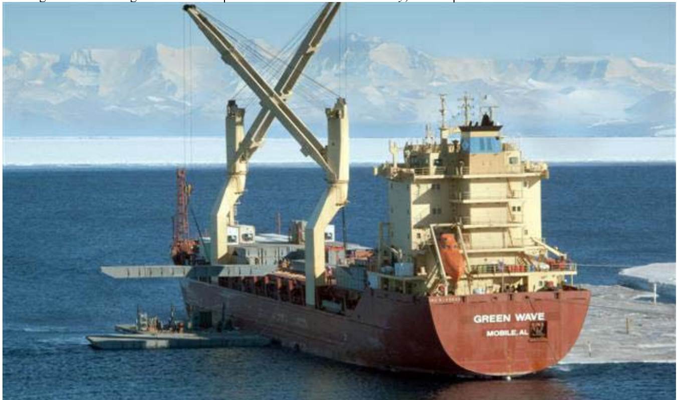
NSF Photo by William Henriksen, 22 February 2012 The annual cargo vessel offloads a metal causeway to be used in lieu of the ice pier at McMurdo Station. Warm temperatures prevented the ice pier from solidifying, so the causeway was used instead.
