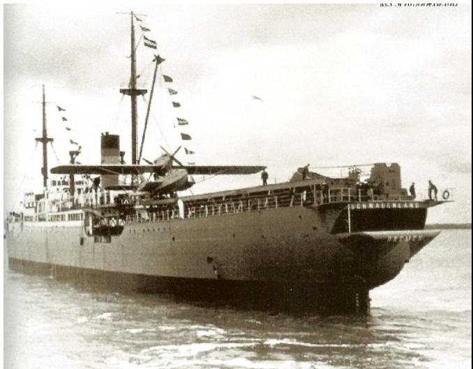
MS Schwabenland , late 1930's, with one of two Dornier flying boats towards the stern which was launched by a steam catapult, on return it would land on the sea and taxi to the ship to be brought aboard by a crane.
