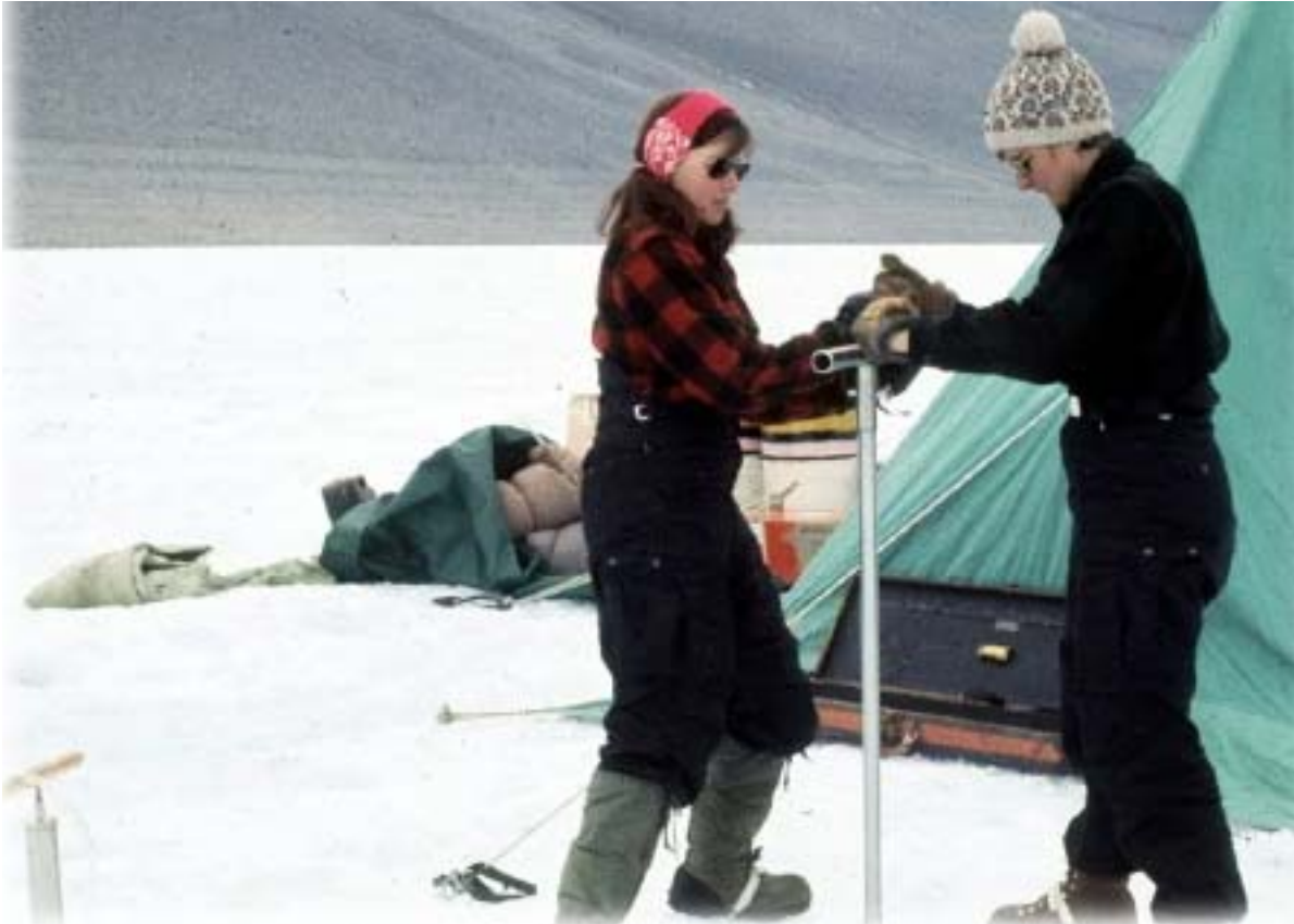
Eileen McSaveney (left) and Terry Tickhill (right) use a hand auger to drill Lake Vanda, Wright Valley, Antarctica, during the 1969–1970 field season. Water collected during this effort was used to date the lake. (photo: Lois Jones via National Science Foundation)
