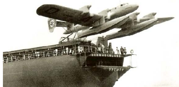
Flying boat being launched by catapult from the Schwabenland for aerial mapping
