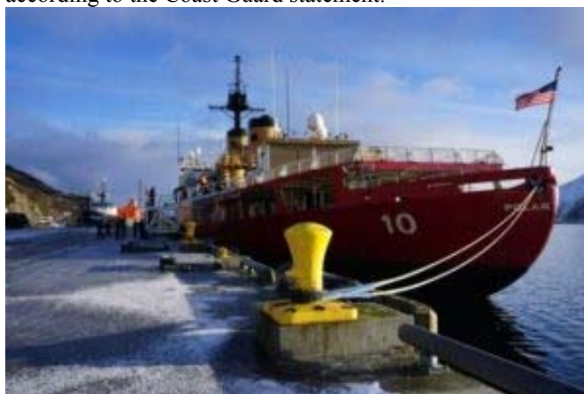
The Polar Star sits in the Port of Dutch Harbor in January 2021. The ship is nearly 400 feet long and can break ice up to 21 feet thick (Hope McKenney/KUCB)
